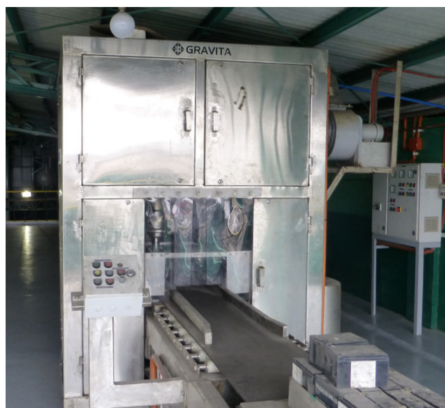
Figure 13: Ventilated battery saw. (Courtesy of Gravita, India)
